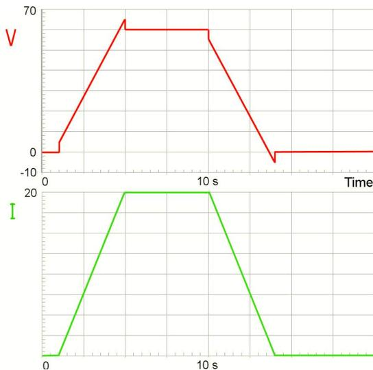
Simulation of operation of a bipolar current controlled power supply (voltage and current vs time)
